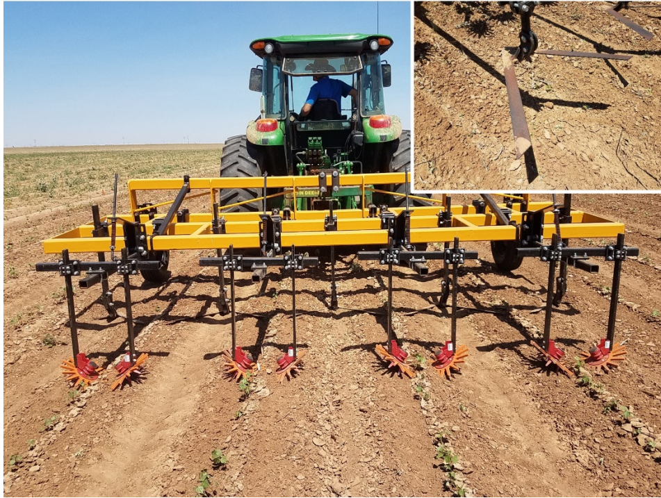
Fig. 1. Cultivator configuration used in Texas A&M studies investigating the use of finger weeders and wide sweeps to control in-row and between-row weeds in cotton. Cultivator design and setup credit: Carl Pepper, Lubbock, TX.
