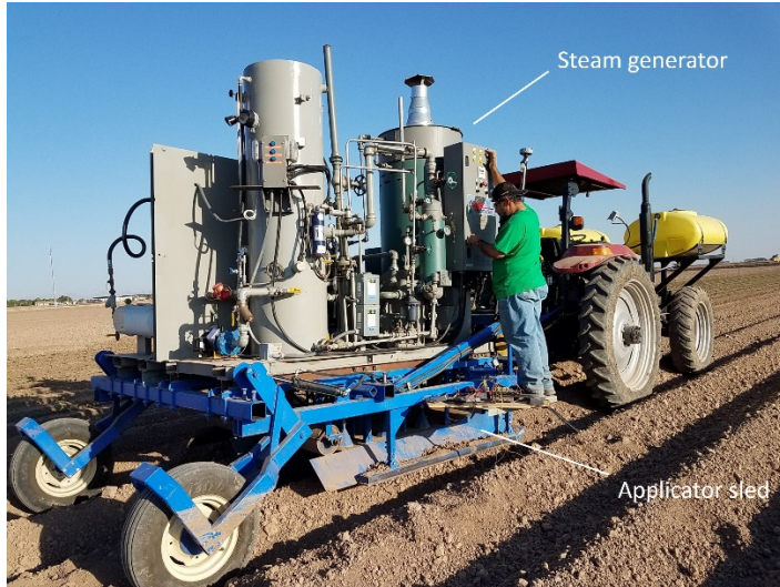
Fig. 1. Band-steam applicator principally comprising a 35 BHP steam generator mounted on a bed-shaper applicator sled.
