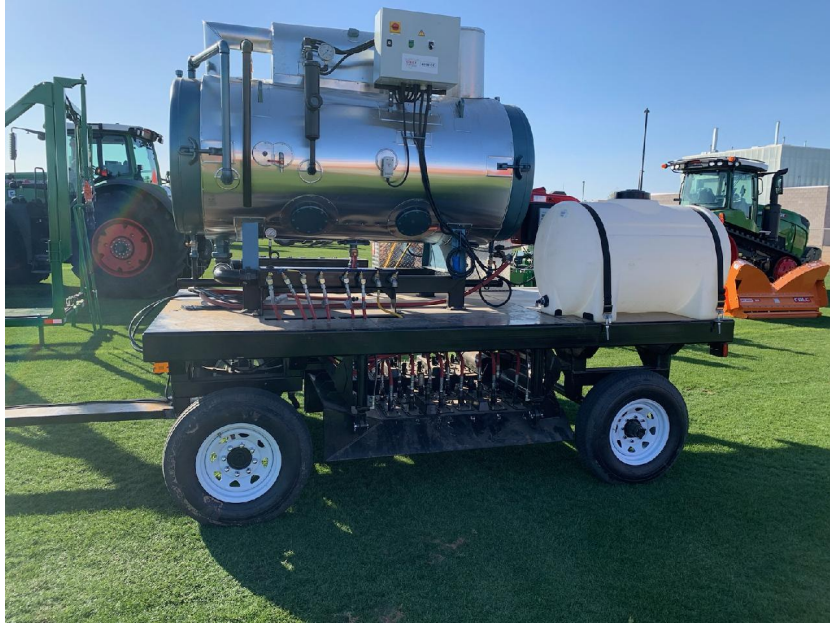
Fig. 1. Prototype band-steam applicator for controlling soilborne pathogens and weeds on display at the 2022 Southwest Ag Summit, Yuma, AZ. Applicator sled and trailer fabricated by Keithly-Williams Fabrication, Yuma, AZ. Steam generator provided courtesy of Simox, Contamine-sur-Arve, France.
