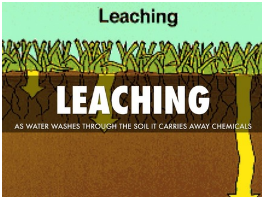
Figure 4. Soil-water leaching process by the movement of gravitational water through a saturated soil.
