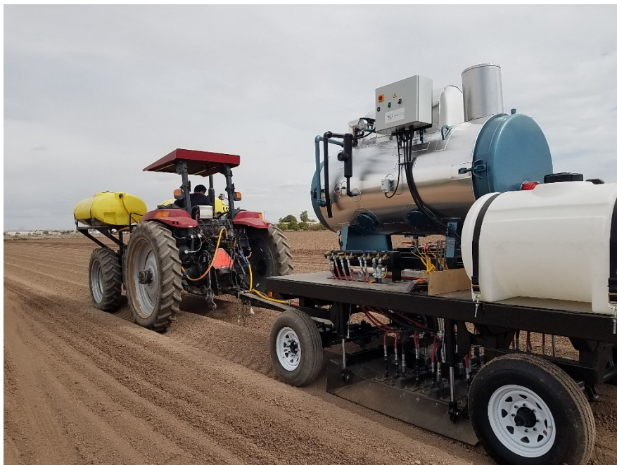
Fig. 3. 2 nd generation band steam applicator to be demoed at the 2023 Southwest Ag Summit Field Demo held February 22 rd , 2023 in Yuma, AZ ( https://yumafreshveg.com/southwest-ag-summit/ ).
